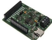
FT231X device supports BCD to simplify and optimize battery charging in portable systems.
