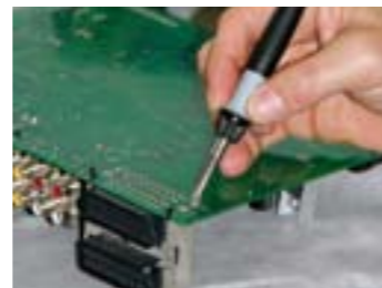
High-mass through-hole soldering with the i-Tool
