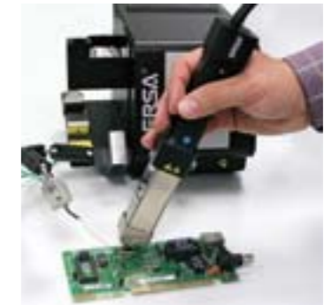
Rapid, simple and safe hand-held component removal
