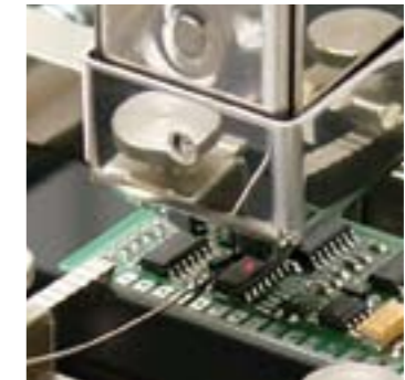
Temperature-controlled SMD soldering
