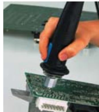
High-mass through-hole desoldering
