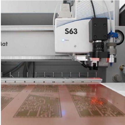
PCB production by milling.
