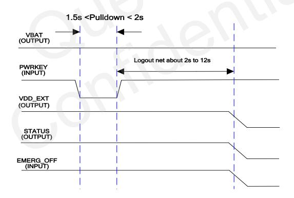
Figure 9: Timing of turning off the module
