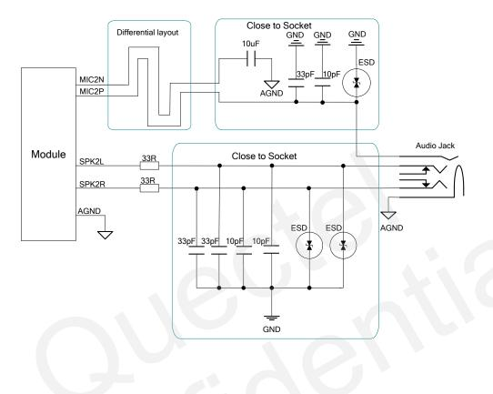
Figure 34: Earphone interface design
