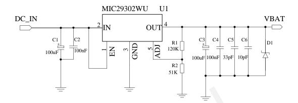
Figure 5: Reference circuit of the power supply input
