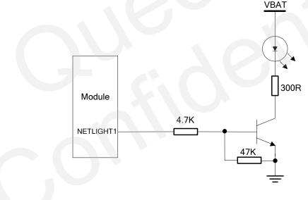
Figure 45: Reference design of the NETLIGHT1
