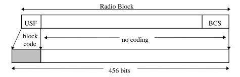
Figure 63: Radio block structure of CS-4
