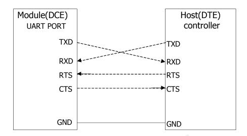
Figure 20: Connection of associated hardware flow control
