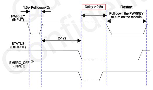
Figure 12: Timing of restarting the system
