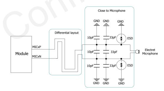
Figure 31: Microphone interface design of AIN1&AIN2
