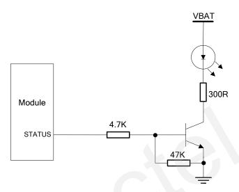
Figure 46: Reference design of the STATUS
