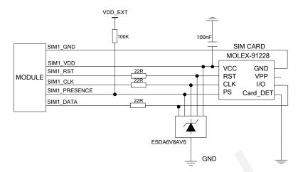
The following figure shows the reference design of the 8-pin SIM card.
