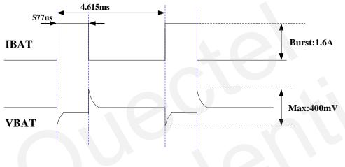
Figure 2: Ripple in supply voltage during transmitting burst
