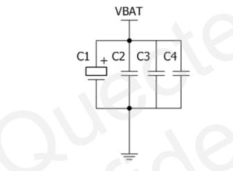
C1>=100uF; C2=0.1uF~1uF; C3=33pF; C4=10pF
