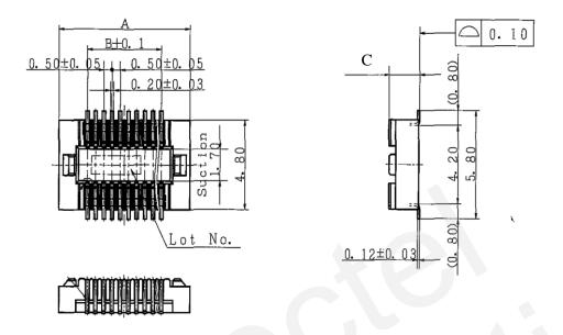
Figure 55: Sketch map of 100 pin board to board socket (Unit: mm)
