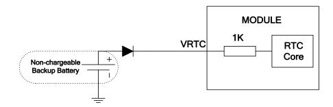
Figure 14: RTC supply from non-chargeable battery
