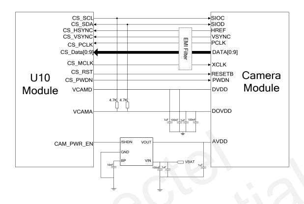
Figure 39: Reference design with digital CMOS sensor
