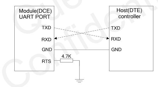
**Figure 19: Connection of three lines UART port**
