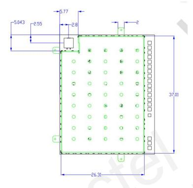
Figure 53: U10 BOT dimension (Unit: mm)
