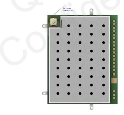
Figure 47: Antenna connector
