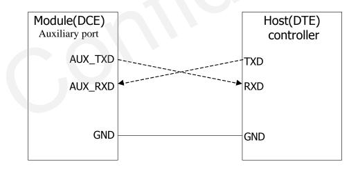
Figure 23: Connection of Auxiliary UART Port
