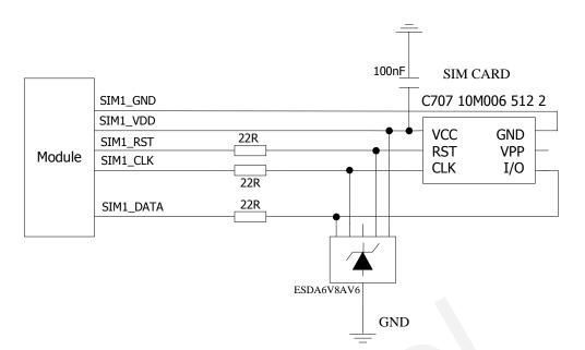
Figure 28: Reference circuit of the 6 pins SIM card
