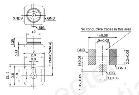
Figure 48: Dimensions of the UF.L-R-SMT connector (Unit: mm)
