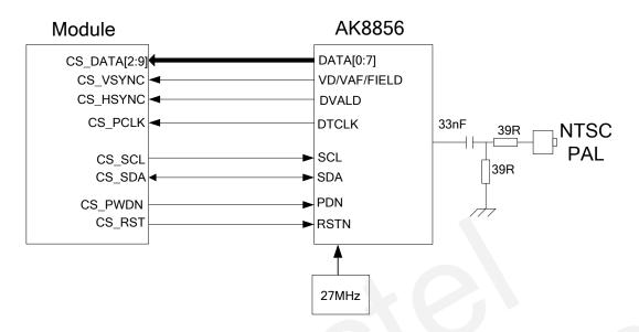
Figure 40: Reference design of using decoder IC for CVBS signal
