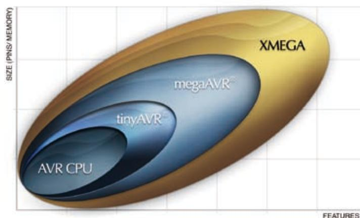
All AVR devices from the smallest tinyAVR to the largest XMEGA uses the same CPU. They differ only in features, pin count and memory size. This enable AVR to cover the complete 8- and 16-bit market with one single, compatible product family.
