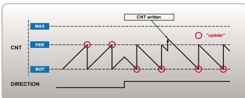
Changing the period with buffering in dual slope mode
