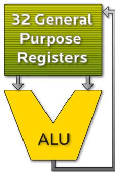
Central in the AVR architecture is the fast-access register file with 32 x 8-bit general purpose working registers directly connected to the Arithmetic Logic Unit. Within a single clock cycle the ALU can be fed two arbitrary registers, do a requested operation, and write back the result.
