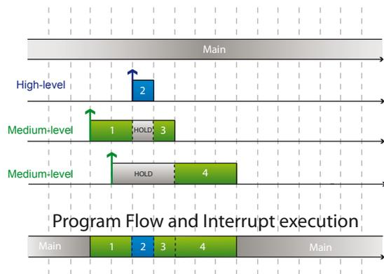
A second interrupt at an interrupt level already being serviced, will pend until the first interrupt routine finishes.
