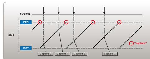
Frequency capture of an external signal
