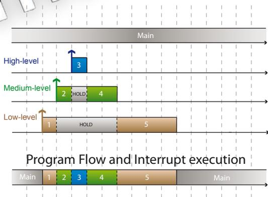
A higher level interrupt will halt execution of a lower level interrupt routine. The lower level interrupt routine will continue and finish after the higher level interrupt routine finishes.
