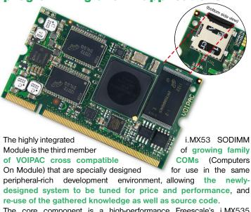
The core component is a high-performance Freescale's i.MX535 advanced multimedia processor with very low power consumption. Only 1mm thick 10-layer HDI micro-via PCB board carries CPU + Flash + SDRAM + Ethernet and provides vast majority of the embedded systems must-have peripherals.
