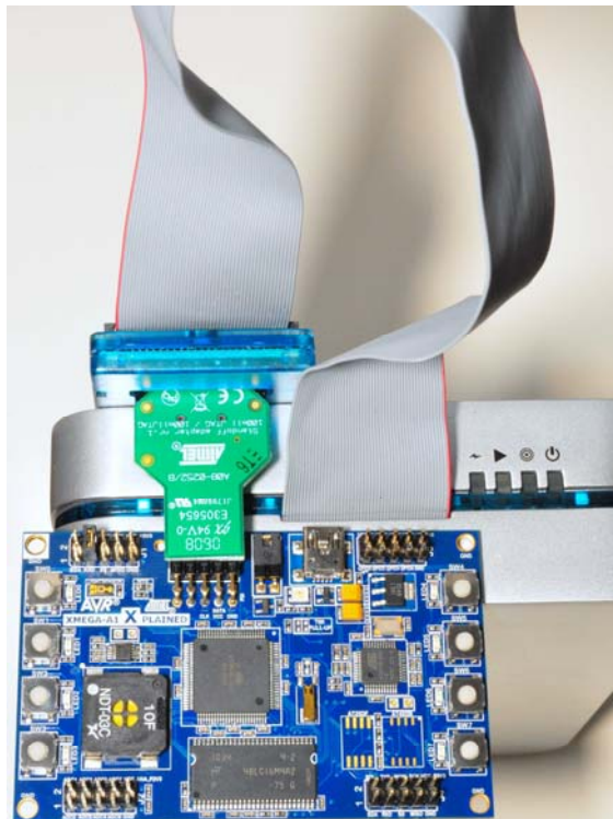
Figure 4-3. Connecting the AVR ONE! debugger to an Xplained board.
