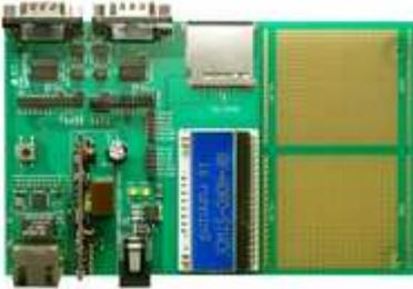
The EVA-Kit can be used to support the integration of the XT-NANO and the XT-NANO-XXL. There are 4 different connection options available. An LCD display, an SD card slot, RS232 and RS485 connections, as well as the option to make available further connections for SPI or I2C over the Wire-Wrap field which is available on the board.
