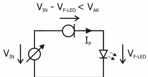
The **CL20M45** is designed for an  $I_P$  of 20mA, which is the typical driving current for Standard LEDs; the  $V_{AK}$  is 45V. So in the easiest case, this CLD can be used to drive a single LED from a voltage source ranging from about **10V<sub>DC</sub> up to 45V<sub>DC</sub>**. For higher driving currents, the **CL40M45** offers an  $I_P$  of 40mA. CLDs can be even operated in parallel; of course then the power dissipation / power losses will increase as well.
