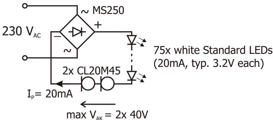
Here the same circuit, but operated at 230V<sub>AC</sub> mains. Due to the higher peak voltage, more LEDs have to be connected in series, and also two CLD are used. Anyway, a single rectifier bridge is enough to complete the whole circuit!
