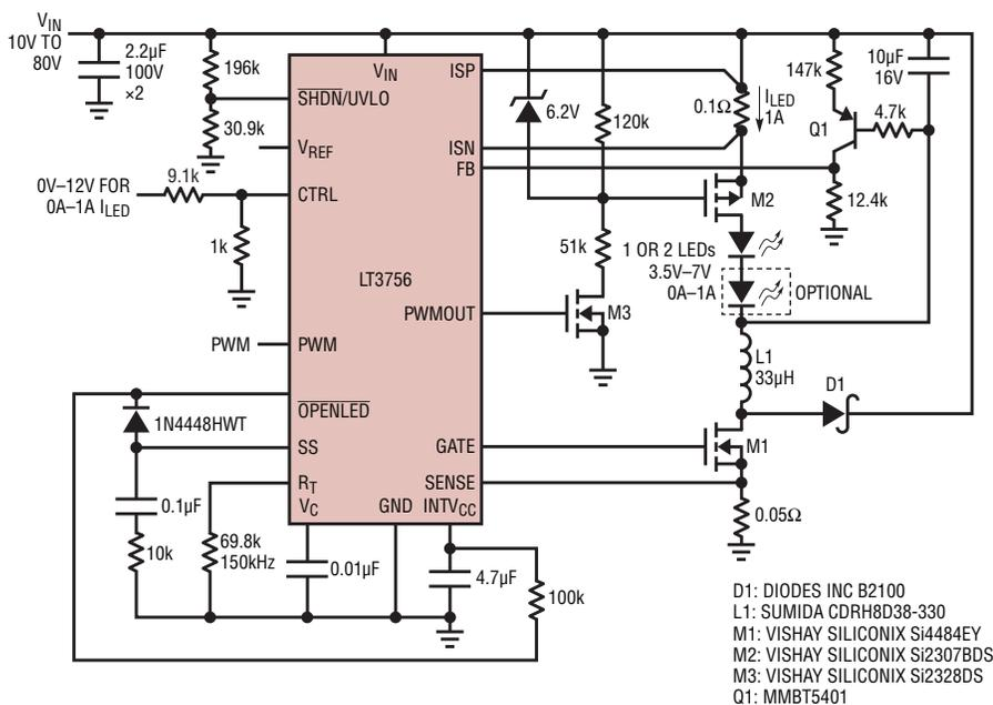
**Figure 2. An 80V<sub>IN</sub> buck mode LED driver with PWM dimming for single or double LEDs**
