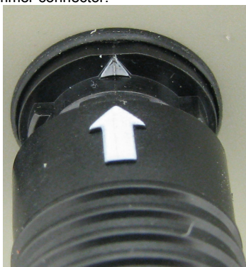
Arrows on power supply connectors
