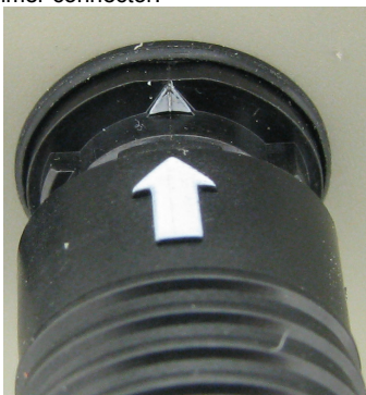
Arrows on power supply connectors
