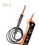
The SN-4 tester is designed for both AC and DC voltage measuring from 110 V to 400 V with frequency up to 60 Hz, detecting of a phase conduc-tor, phase sequence of three phase system with a neutral wire and detecting polarity of DC voltage.
